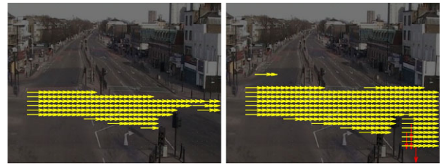
Fig. 9 Example of fine grained cluster decomposition discovered: strictly horizontal vs. turning flows
