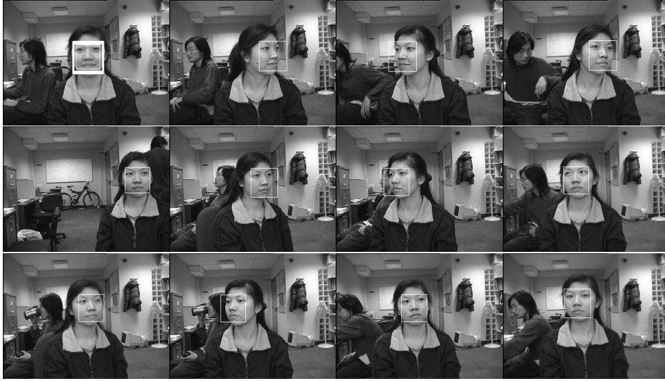
Figure 4: Experiment 2 - Tracking a non-frontal female face in real-time with the proposed objective function. The figure shows example images from an indoor sequence (Video Sequence 1).
