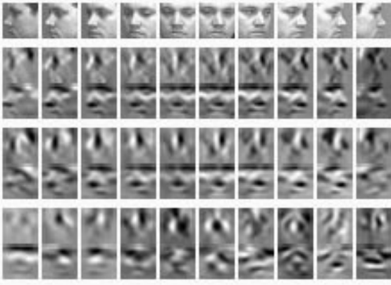
Figure 2. Representation for pose estimation. From top row to bottom row are the original face images, the corresponding filtered patterns, reconstructed patterns from the first 20 PCs, and the first 10 significant PCs.
