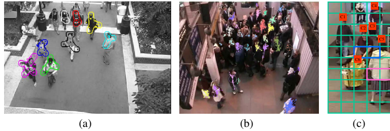
Fig. 3 (a) and (b) show the results of clustering coherent motions using methods proposed in [63] and [7] respectively. (c) shows the pairwise affinity of patches (strong affinity = magenta, weak affinity = blue) in terms of motion and colour constancy; the affinity is used to determine the assignment of patches to person hypotheses [77]. Images from [7, 63, 77].
