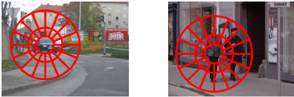
Figure 1. Examples of the polar geometric structure. The target object classes are car and people respectively in the left and right images.
