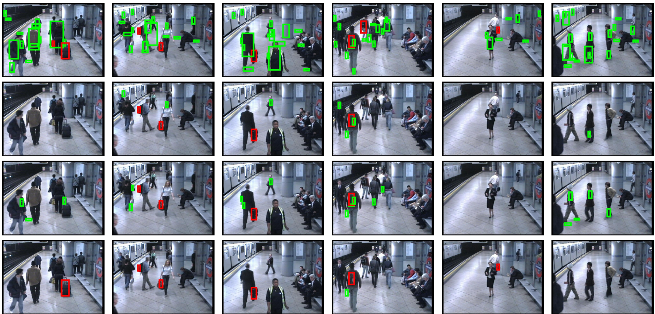
Figure 5. Compare examples of object detections using HOG, TAS and MMC models on i-LIDS. The first row corresponds to results from HOG without threshold. The second, third and fourth rows correspond to HOG, TAS and MMC with threshold respectively. The red bounding box indicates true positive detections and the green one is for false positives.
