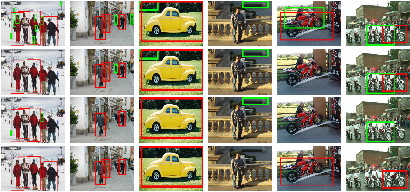
Figure 4. Compare examples of object detections using HOG, TAS and MMC models on PASCAL. The left-hand side two columns are for people detection, the middle two are for car detection, and the right-hand side two are for motorbike detection. The first row corresponds to results from HOG without threshold, the second, third and fourth rows correspond to HOG, TAS and MMC with threshold respectively. The red bounding box indicates true positive detections and the green one is for false positives.
