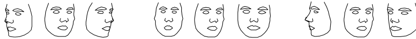
Figure 6: First three modes of shape variation for a Kernel PCA based PDM. The range of variation is set to -1.5\sqrt{\lambda_i} \leq b_i \leq 1.5\sqrt{\lambda_i} .
