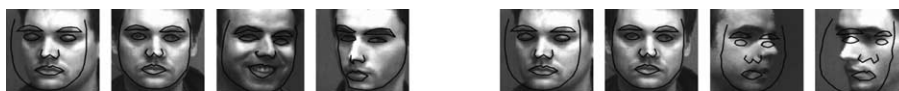
Fig. 8. Fitting shapes to images using linear ASMs trained across \pm 20^\circ (left) and \pm 90^\circ (right).
