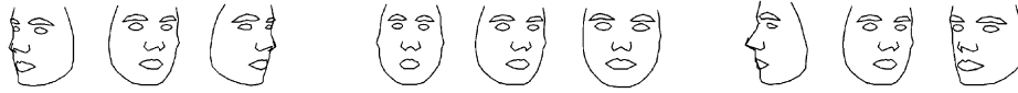
Fig. 9. First three modes of shape variation for a KPCA based non-linear PDM. The VSR was set to -1.5\sqrt{\lambda_i} \leq b_i \leq 1.5\sqrt{\lambda_i} .
