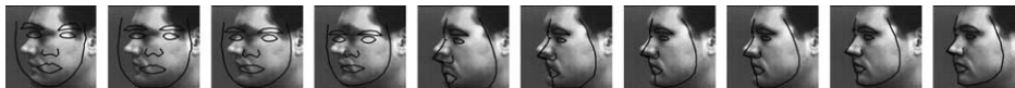
Fig. 12. An example of fitting a shape to a face image and recovering its pose at -80^\circ . The estimated shapes overlaid upon the images are shown after iterations 0, 1, 4, 6, 12, 13, 15, 16, 20 and 25.
