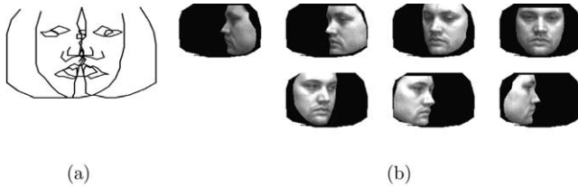
Fig. 5. (a) A generic-view shape template is based on aligning shapes from two profiles and the frontal view with respect to a single or a set of inner landmarks. (b) Examples of aligned appearances of both shape and texture at different poses using just one inner landmark assigned to the nose-tip.
