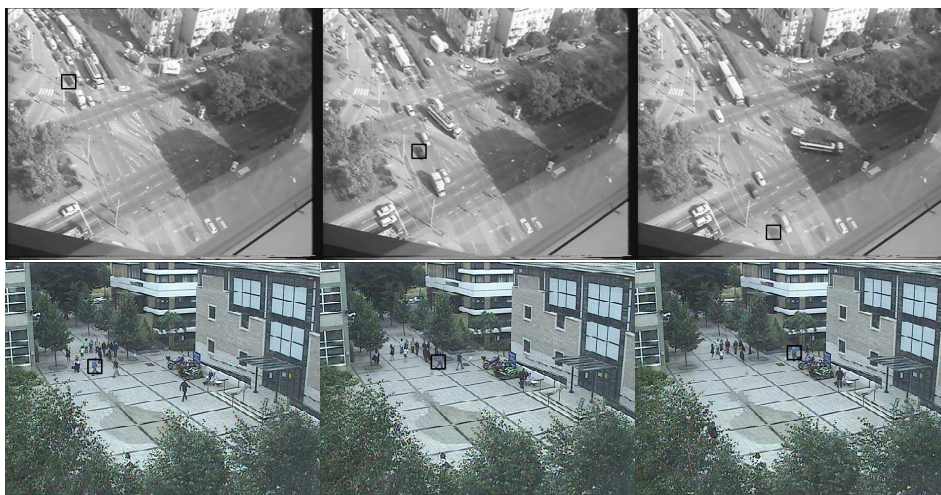
Figure 6: A car on a busy road is tracked in Experiment 11 and a pedestrian is tracked in Experiment 12. It is shown that the tracker combined with non-uniform sampling for arbitrary spatial weighting tracks the car and the pedestrian successfully.
