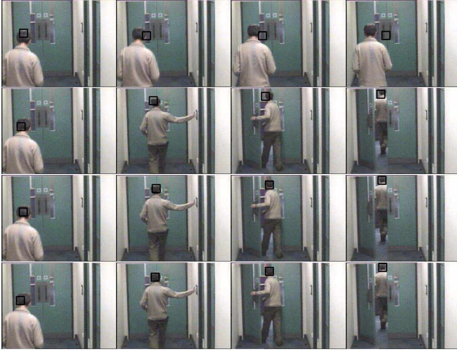
Figure 2: Experiments 5, 6, 7 and 8: The four rows of images represent four separate video sequences produced by four experiments respectively. In Experiment 5 (first row), only 2 random samples are picked from each of the candidate and model images, 3 samples in Experiment 6 (second row), 5 samples in Experiment 7 (third row) and all samples from the candidate and model images (traditional Mean-Shift Tracking) in Experiment 8 (fourth row).
