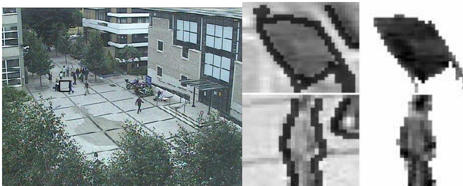
Figure 7: In the left image, Experiment 12 is repeated without non-uniform sampling for arbitrary spatial weighting. The original mean-shift tracker fails to track the pedestrian. The right image shows that the spatial distributions of the pixels from the objects (Experiment 11 and Experiment 12) extracted by Normalized Cut are used to build 2-dimensional histograms for the estimate of the spatial importance, \hat{\delta}(\mathbf{x}) .
