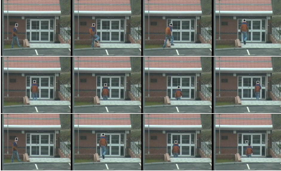
Figure 3: In Experiment 9 (first two rows), the black hat of a person against a red wall and a glass door as the background is tracked. It is shown that the tracker combined with our on-line feature selection method tracks the black hat successfully when the hat moves in front of a glass door outside a dark corridor. In the bottom row, Experiment 9 is repeated without on-line feature selection. The original mean-shift tracker is distracted by the glass door on the background.
