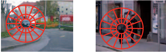
Fig. 3. Examples of the polar geometric structure for context modelling. The target object classes are car (left image) and people (right image).
