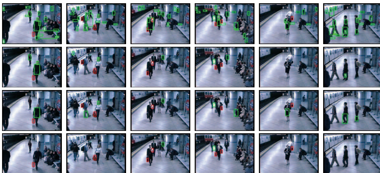
Fig. 10. Examples of object detections using HOG, TAS and MMC models for luggage detection on i-LIDS.
