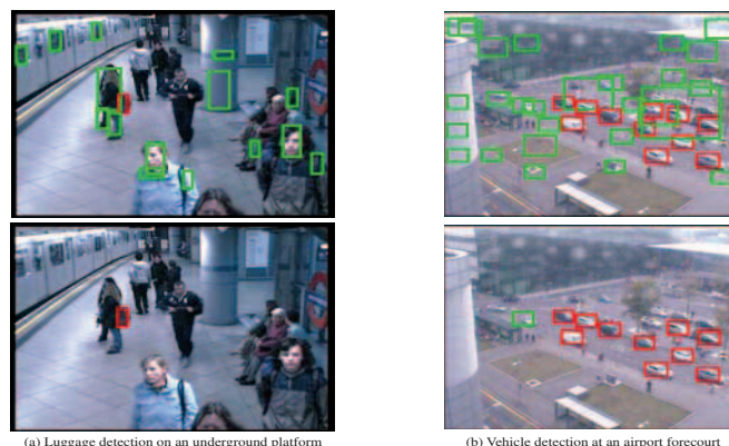
Fig. 1. Examples of improving object detection using contextual information. The top row shows the detection results by a HOG detector [12] without context modelling, and the second row shows the results obtained by using the same detector with the proposed context model. The green and red bounding boxes indicate false detections and true detections respectively.
