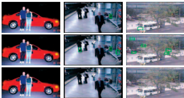
Fig. 12. Examples of failed detections. The first, second and third rows correspond to results of HOG, TAS and MMC with threshold respectively. The green bounding box shows false positive detections.
